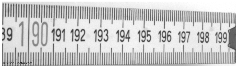
Fig. 5: Stop-downed lens, large depth of field, uniform expansion of the depth of field towards the camera / away from the camera:
